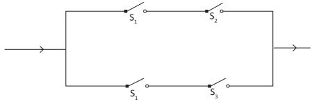
There is a flow of current in the circuit if and only if  $S_1$  is closed and either  $S_2$  is closed or  $S_3$  is closed.
