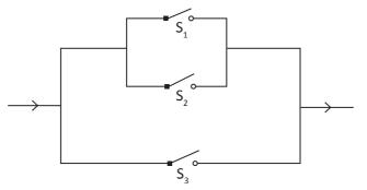
The current flows in the circuit if both  $S_1$  and  $S_2$  are closed or  $S_3$  is closed.
