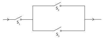
There is a flow of current in the circuit if and only if  $S_1$  is closed and either  $S_2$  is closed or  $S_3$  is closed.
